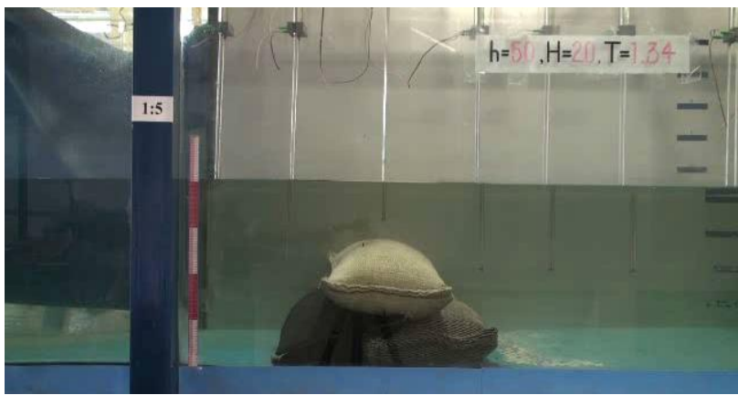
Laboratory modeling of wave energy mitigation by submerged breakwaters
